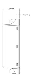
NOTE: Unit size: mm[inch] Terminal tolerance: ±0.1mm Unmarked tolerances: ±0.5mm
